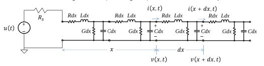
$$v(x + dx) = v(x,t) - Ri(x,t)dx - L\frac{\partial i(x,t)}{\partial t}dx$$
