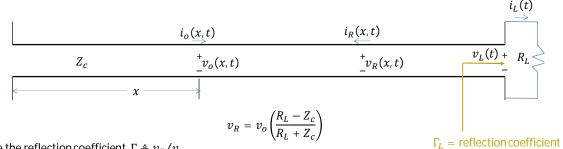
Define the reflection coefficient,  $\Gamma \triangleq v_R/v_o$
